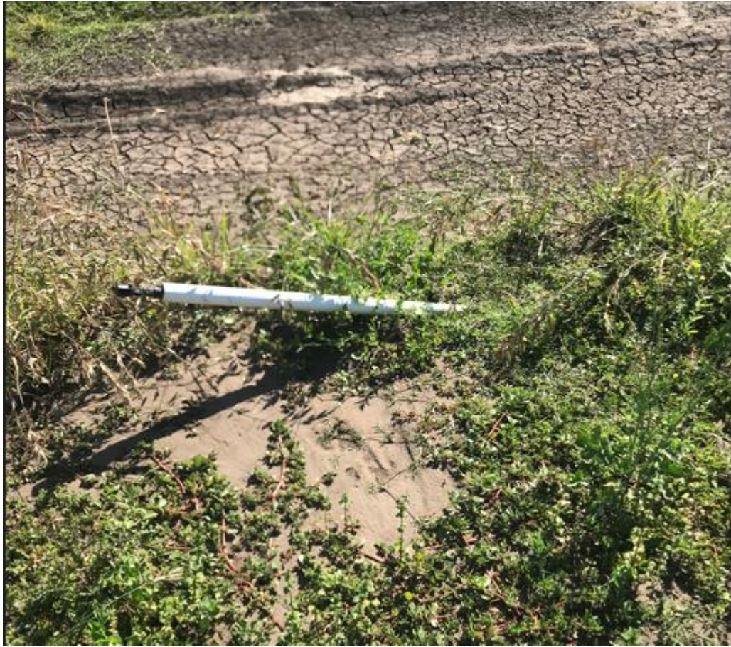
Above & below: Broken irrigation upright to be reconnected to underground piping
