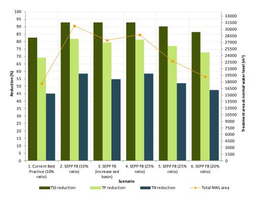
**Figure 2.** Pollution reductions and required treatment areas for each scenario with an extended detention depth of 0.35 m. Scenario 1 represents current design arrangement.
