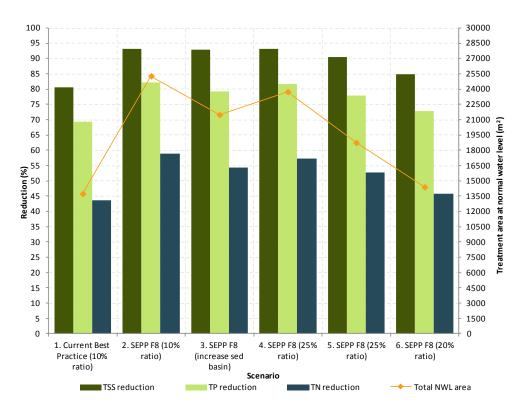
Figure 3. Pollution reductions and required treatment areas for each scenario with an extended detention depth of 0.5 m
