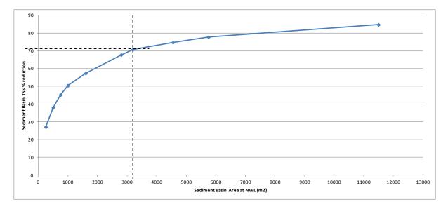
Figure 4. Sediment basin diminishing performance based on control catchment and EDD of 0.35
