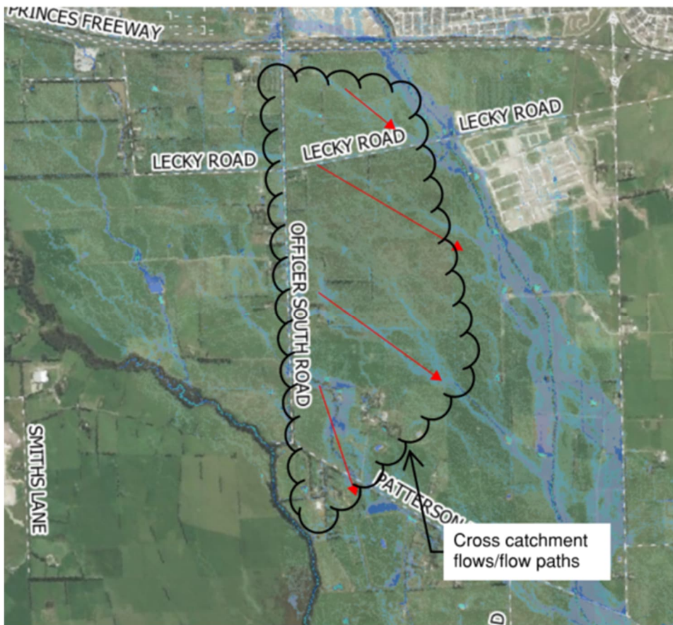
Figure 9-2: Overland flow paths and diversion downstream of the Princes Freeway (1% AEP example)
