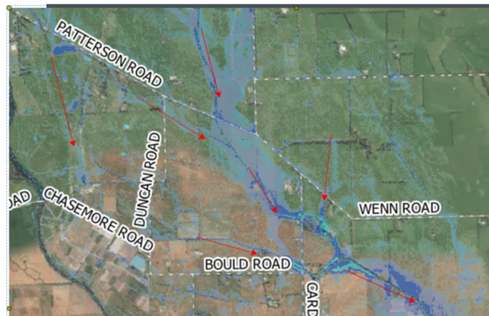
Figure 9-2: Overland flow paths and diversion downstream of the Princes Freeway (1% AEP example)
