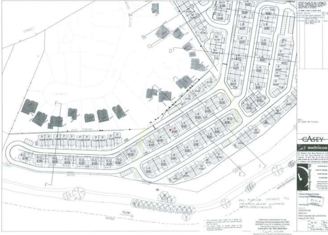
Figure 40: Endorsed plans showing the locations of proposed dwellings at Rivervue Retirement Village, including finished floor levels. The sections identified in this plan are shown in Figure 39.
