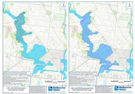
Figure 49: Comparison of the estimated extent of the Flood Event, which included the Floodwall (left panel) and the extent of the modelled extent of the Flood Event, which did not include the Floodwall (right panel).
