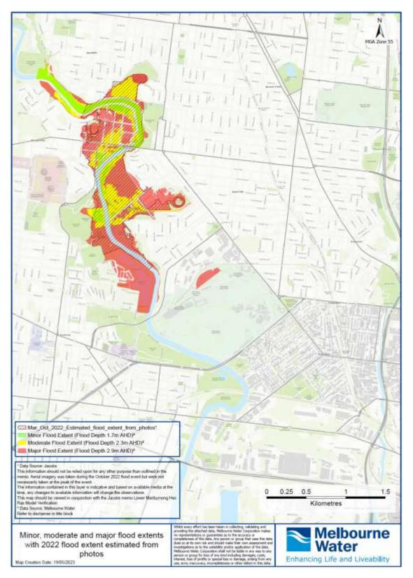
Figure 5: Spatial extent of flooding in the lower Maribyrnong River between Aberfeldie Park and Thomson Reserve resulting from the Flood Event, showing classification of flood extent. (Source: Jacobs, 2023, Lower Maribyrnong HEC-RA Model Verification\_RevB).
