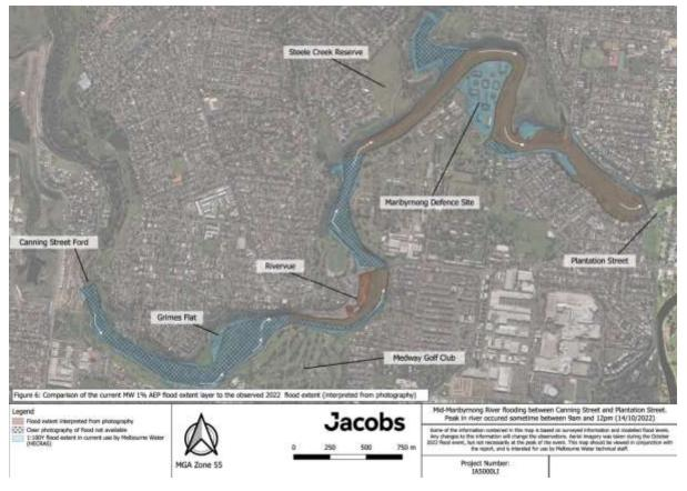
Figure 6: Spatial extent of flooding in the mid Maribyrnong River between Canning Street and Plantation Street resulting from the Flood Event. (Source: Jacobs, 2023, Mid Maribyrnong HEC-RAS Model Verification RevB).
