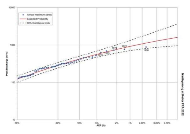
Figure 32: Results of calibration of Maribyrnong RORB model. (Source: Produced by the Panel using data from Jacobs (2023) Maribyrnong Flood Event October 2022 – Post event analysis).
