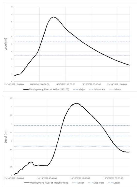
Figure 28: Flood hydrographs for the October 2022 event at Keilor and Maribyrnong gauges showing the duration above minor, moderate and major flood levels.(Source: Produced by the IRP based on information provided).
