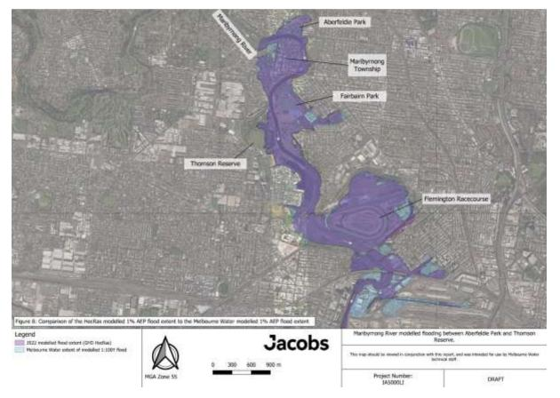
Figure 33: Comparison of modelled spatial extents of the Flood Event and the 1% AEP flood for the lower Maribyrnong model.
