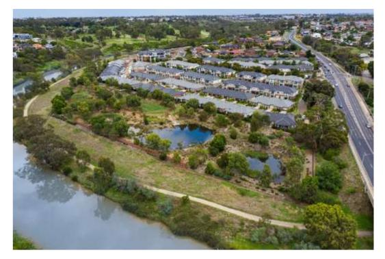
Figure 10: Photo of Rivervue Retirement Village (prior to the Flood Event), showing the constructed retarding basins in the area of the site close to the river corridor land. Canning Street is seen at the right of photo. (Source: Submission #44).
