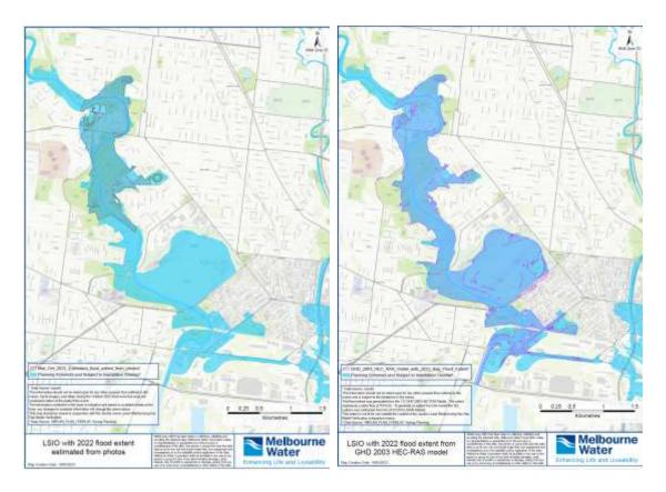
Figure 35: Comparison of the extent of the Flood Event estimated from photos and the 1% LSIO (left panel) and of the extent of the Flood Event estimated using the lower Maribyrnong HEC-RAS model and the 1% LSIO (right panel).
