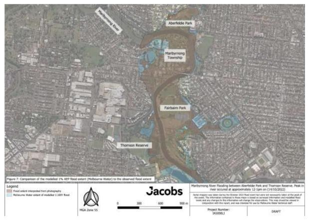
Figure 34: Comparison of estimate actual spatial extent of the Flood Event and modelled spatial extent of 1% AEP flood for part of the lower Maribyrnong model. (Source: Jacobs (2023) Lower Maribyrnong HEC-RAS Model Verification RevB).
